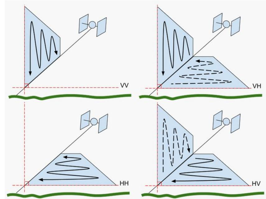
Figure 2: SAR signals are transmitted and received either vertically (V) or horizontally (H). This gives the potential for four different polarization combinations (transmit listed first, receive second): VV, VH, HH, and HV. Credit: ASF
