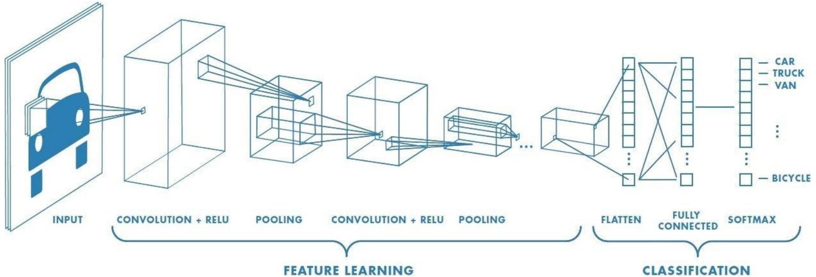
Uses convolution and pooling operations
